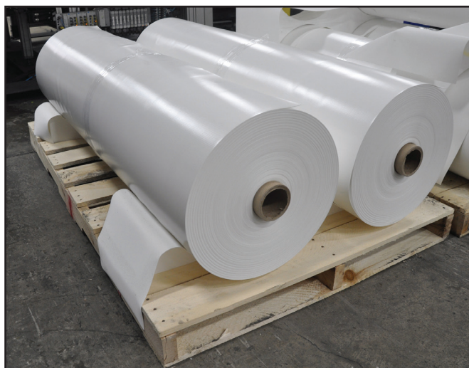
Single-ply roofing membrane is known in the industry to have a very robust life cycle. But it took an NSF/ANSI standard created to document those facts.
